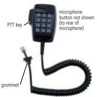
The microphone button operates a hookswitch, which is closed when the microphone is connected to the microphone clip and open when the microphone is removed from the microphone clip. The function of the hookswitch is determined by the radio programming.
